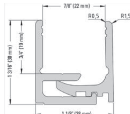
For glass thicknesses 9/16" - 11/16" (15 - 17.52 mm), 1/8" (3 mm) setting block, BO 51 210 03
